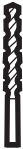
3/8" Drill Bit (If installing into fiberglass ducting with toggle bolts (not included))
